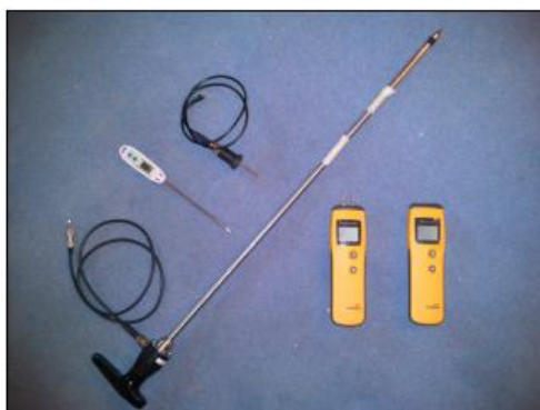
Figure 6 Timbermaster, Balemaster, Balemaster Probe, Digital Thermometer and Thermocouple (Robinson, 2014)
