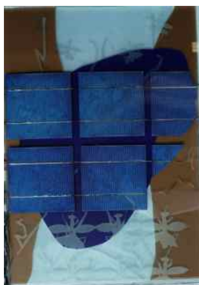
Figure 2: (Left) Artwork incorporating PV in a standard array, with cells positioned perpendicular to incoming light; (Right) LSC-based artwork, with PV strip cells glued to the edges of fluorescent PMMA, to receive light transmitted by total internal reflection.
