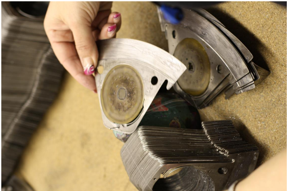
Inserting 'threading' bobbins into their carriages, Cluny Lace, 2013 (picture credit: Julie Botticello)
