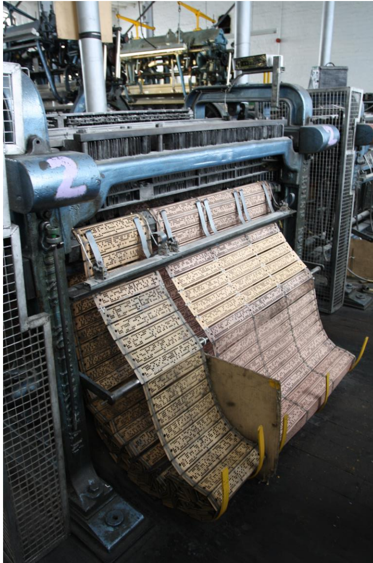
Jacquard cards that control the movement of the threads in the Leavers Machine, Cluny Lace, 2013. (picture credit: Julie Botticello)
