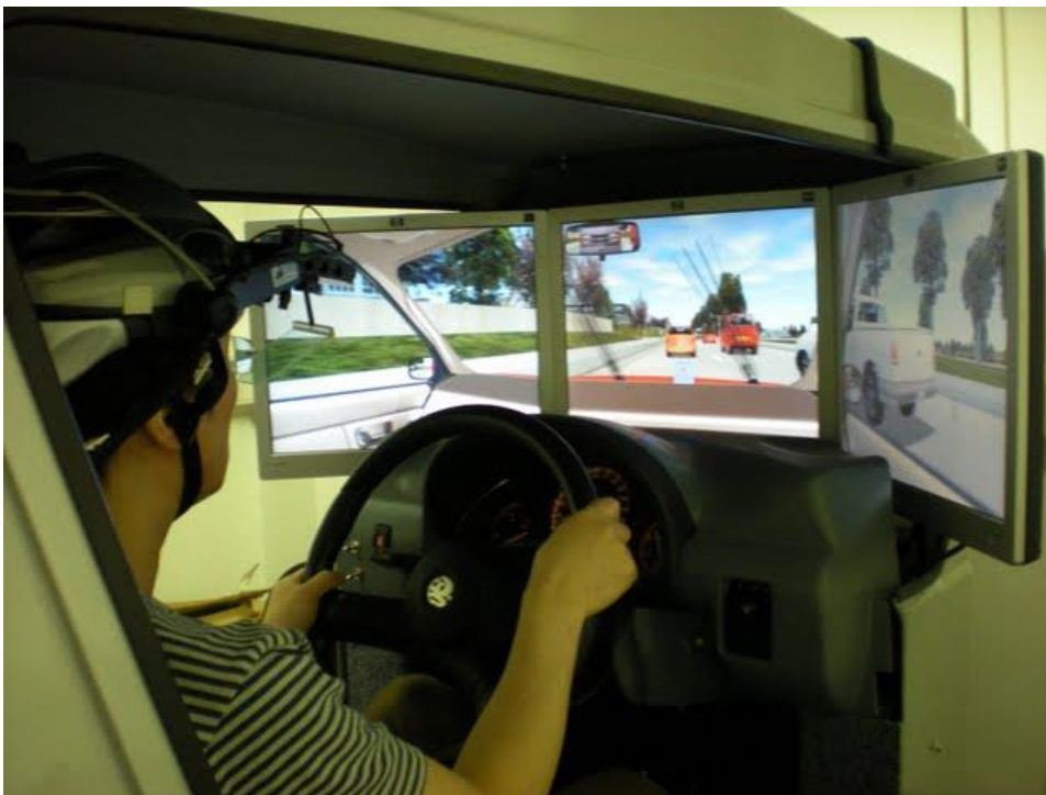
Figure 1. Simulator and SMI head-mounted eye tracker. The figure shows the view in the wide screen condition.
