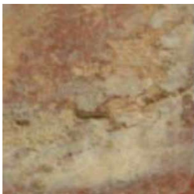
Figure 2. Colour digital images captured with PRISMS from the 12th C wall painting in Plumpton Church, Sussex showing a crack and the surface of the wall. The image is of a region \sim 1.5 cm \times 1.5 cm taken from a distance of 6 m
