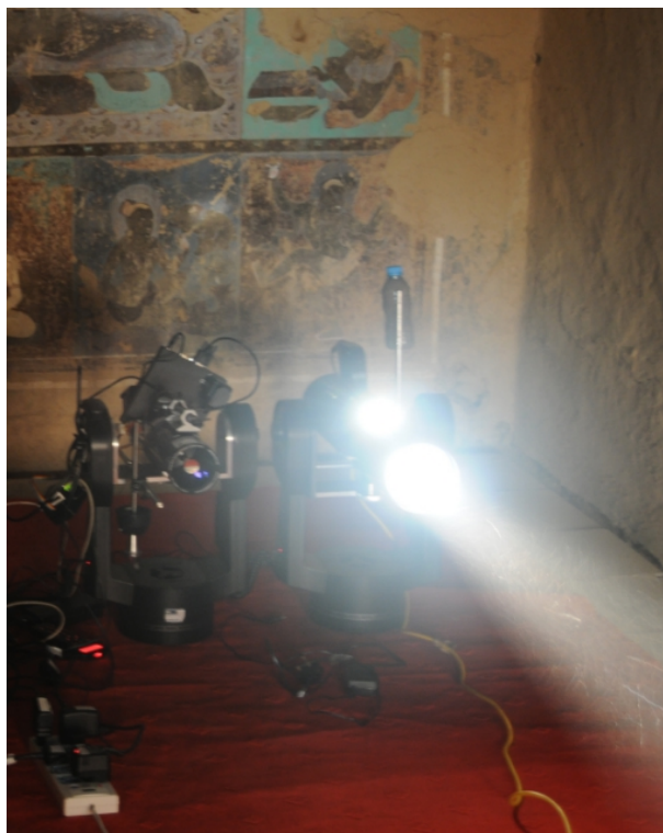
Figure 3: The spectral imaging system PRISMS in cave 465 of Mogao caves, Dunhuang. The imaging system is on the left of the lighting system.
