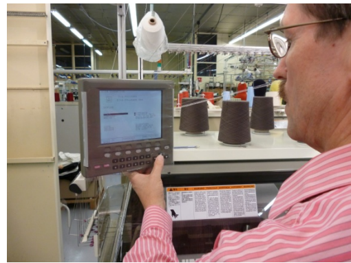
Figure 9: Using the workstation to re-program the knitting machine
