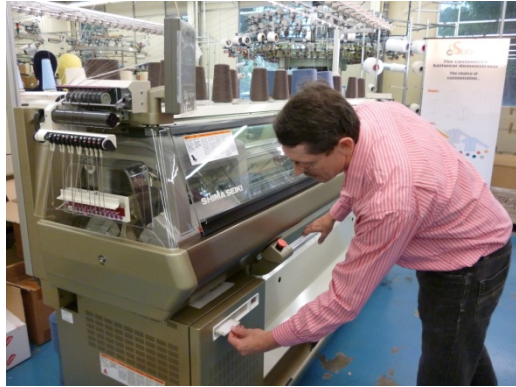
Figure 8: Re-programming the knitting machine with floppy disk
