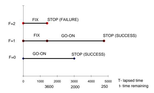
Figure 4: The optimal testing policy for the first numerical example
