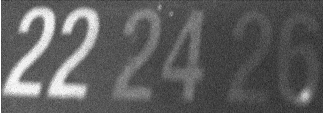
Figure 7. A photograph of a liquid crystal thermometer immediately after being irradiated with the microfademeter. Note 22 is clearly visible at 22°C room temperature and the bottom right hand corner of the 26 showing a small circular area which has been increased in temperature to approximately 26°C by the focused probe.
