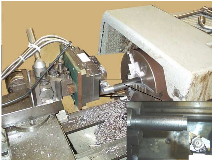
Figure 3: A schematic diagram of the experimental set-up using a force dynamometer.
