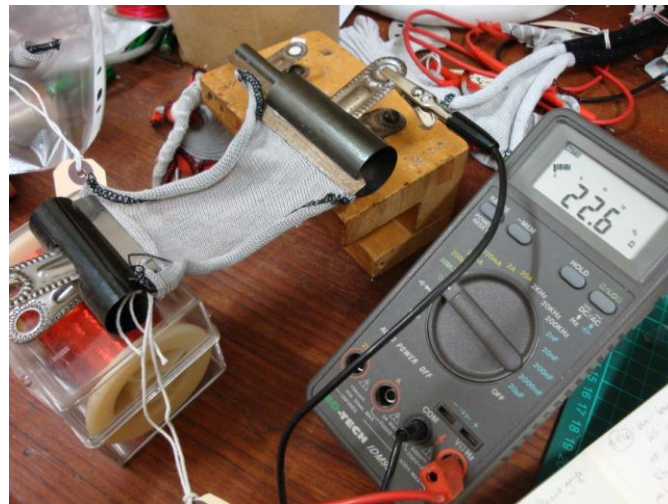
Figure 10: electronic testing of knitted stretch sensor
