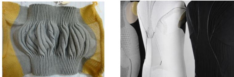
figure 1, left: knitted stretch sensor sample with steel yarn
