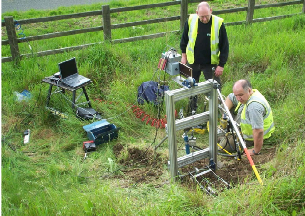
Figure 3. In situ shear and root pull out apparatus developed at Nottingham Trent University (Norris, 18 ).
