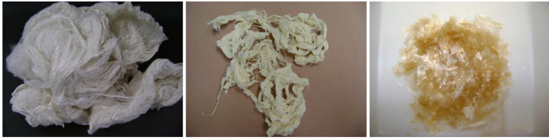
Figure 1. Condition of silk a). After degumming b). Formic acid insoluble c). Formic acid soluble.
