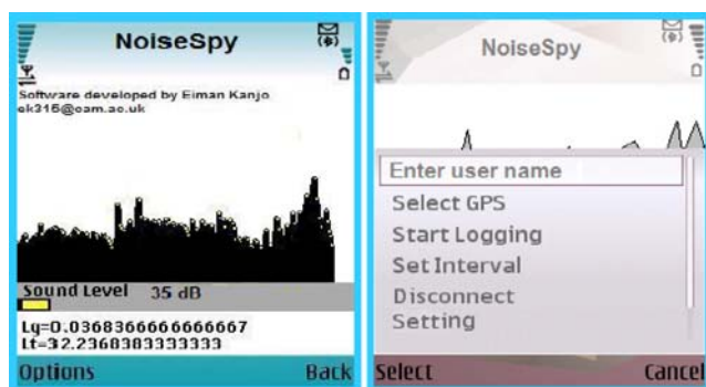
Fig. 5 The first form of on device visualization where the user sees a data/time graph while collecting data
