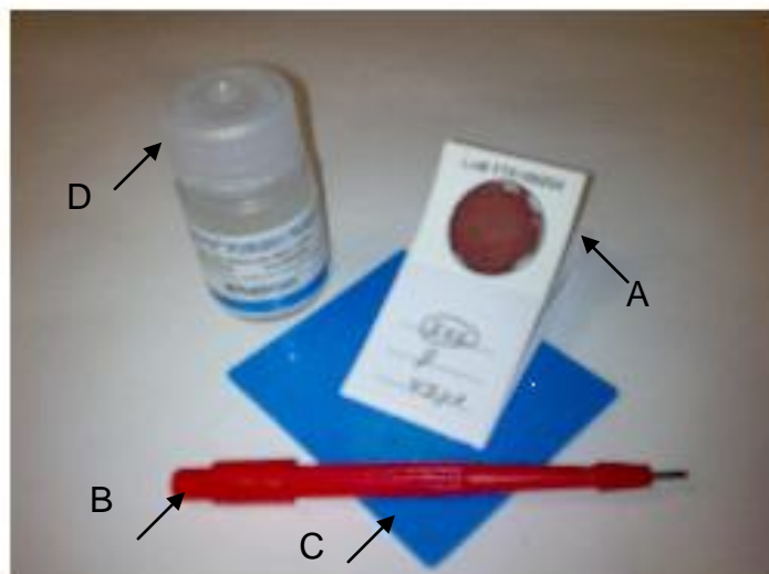
Figure 2.1: Whatman FTA kit. A is a whole blood sample on FTA micro-card (Cat.No.WB120310), B is a Harris Uni-Core Micro-Punch with 1.2 mm steel tip (Cat. No. WB1000028), C is a cutting mat, and D is the FTA Purification Reagent.
