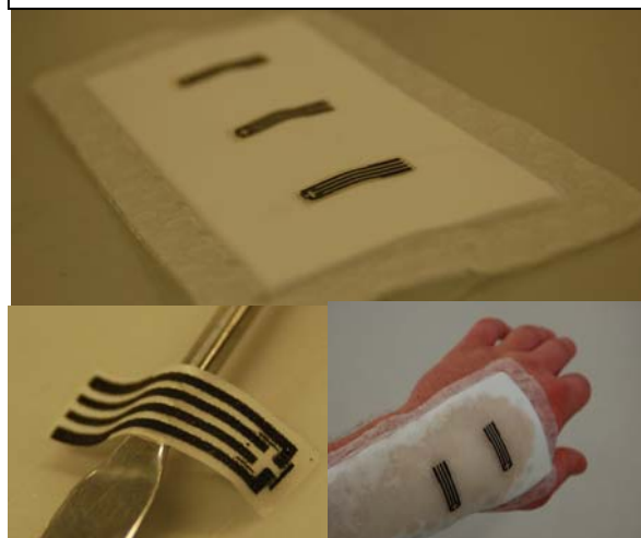
Figure 1.4. Prototype smart-bandage manufactured using pad-printed sensor technology
