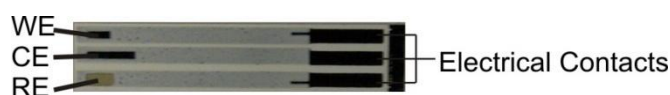
Figure 10.1 The electrode assembly – working electrode (WE), counter electrode (CE) and reference electrode (RE).
