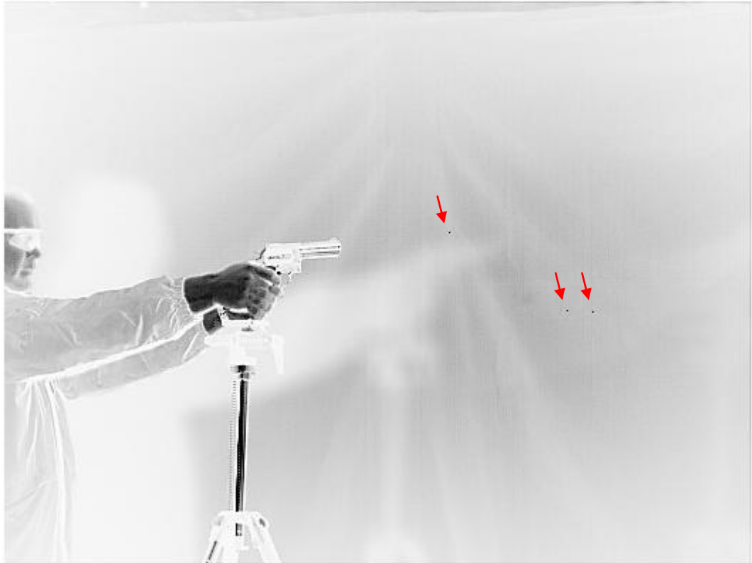
Figure 37: Inverted black and white freeze frame from fast video recording of revolver discharge. Small particles of partially burnt/unburned particles are highlighted with red arrows (particle locations enhanced for printed version).
