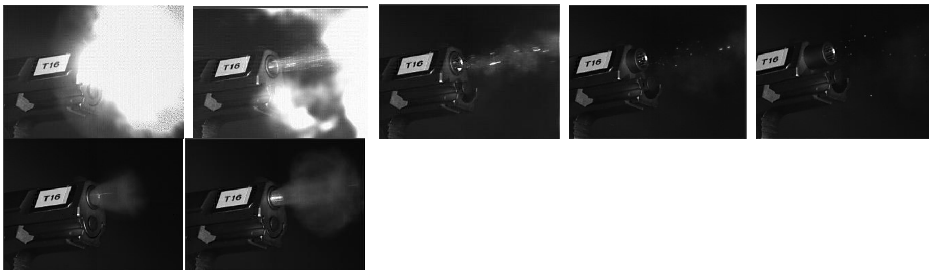
Figure 41: still frames taken from fast video footage of a Walther P99 discharge (very close framing). Settings of the fast video equipment were; frame rate 30000 fps, exposure time 100usec.
