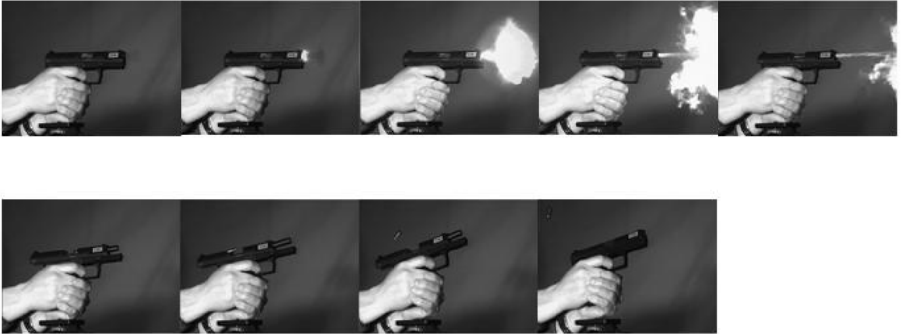
Figure 40: still frames taken from fast video footage of a Walther P99 discharge (close framing). Settings of the fast video equipment were; frame rate 10000 fps, exposure time 100usec.
