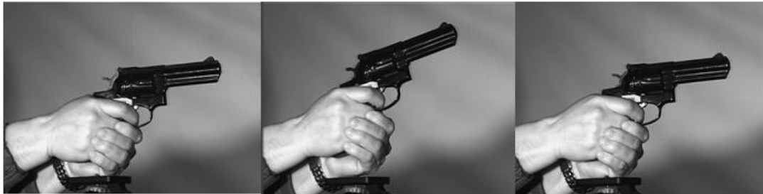
Figure 35: Still frames taken from fast video footage of a revolver discharge. Settings of the fast video equipment were; frame rate 10000 fps, exposure time 100usec total record time 3604 frames.
