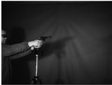
Figure 36: Still frames taken from fast video footage of a revolver discharge (wider framing). Settings of the fast video equipment were; frame rate 10000 fps, exposure time 100usec.
