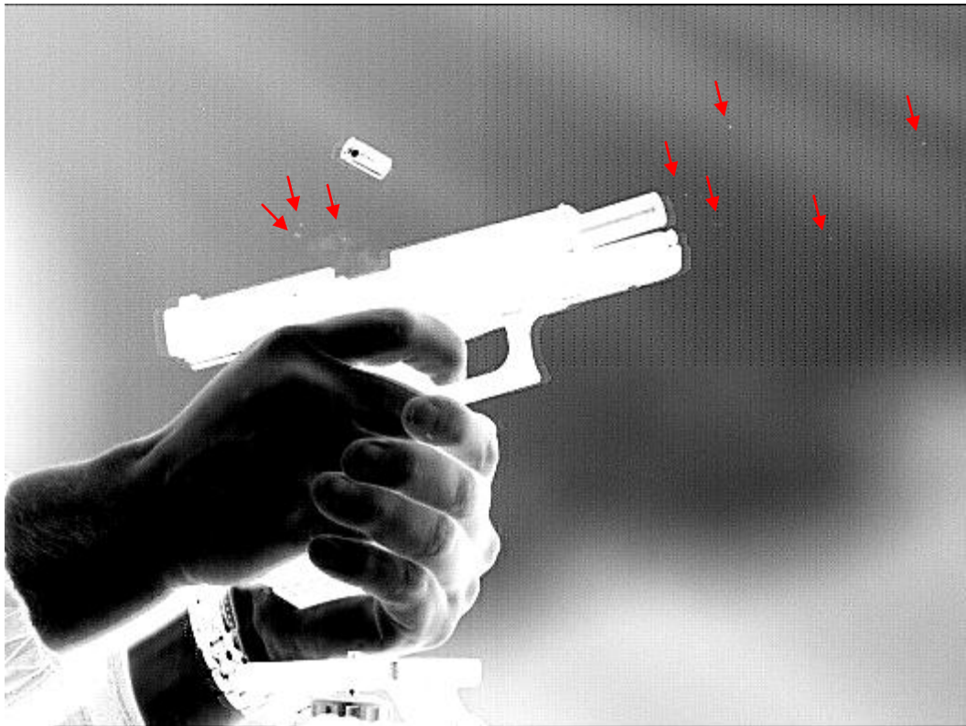
Figure 39: inverted black and white freeze frame from fast video of Glock 26 discharge. Particles of propellant materials are highlighted with red arrows.
