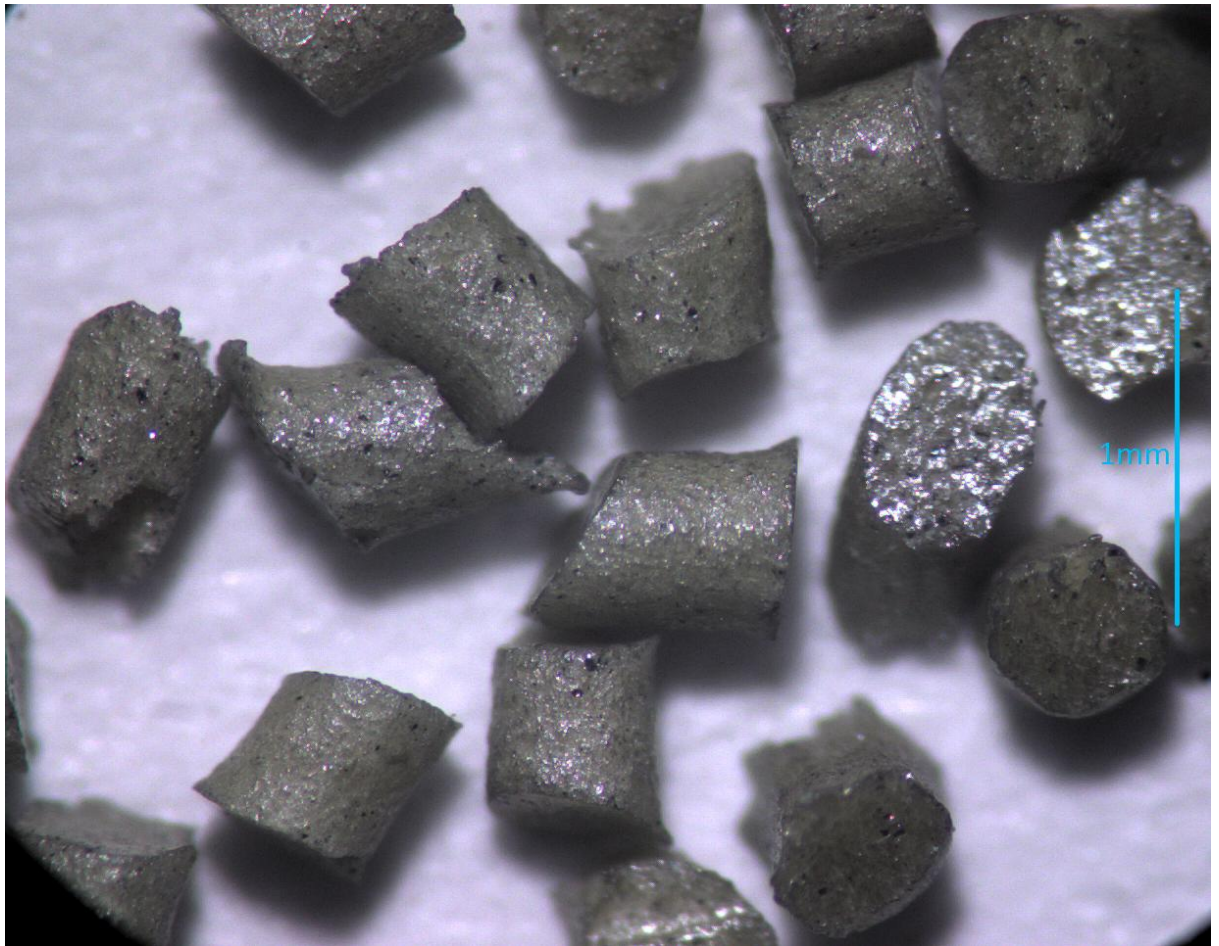
Figure 49: Macroscopic image of Geco .38spl unburned powder. 30 x magnification.
