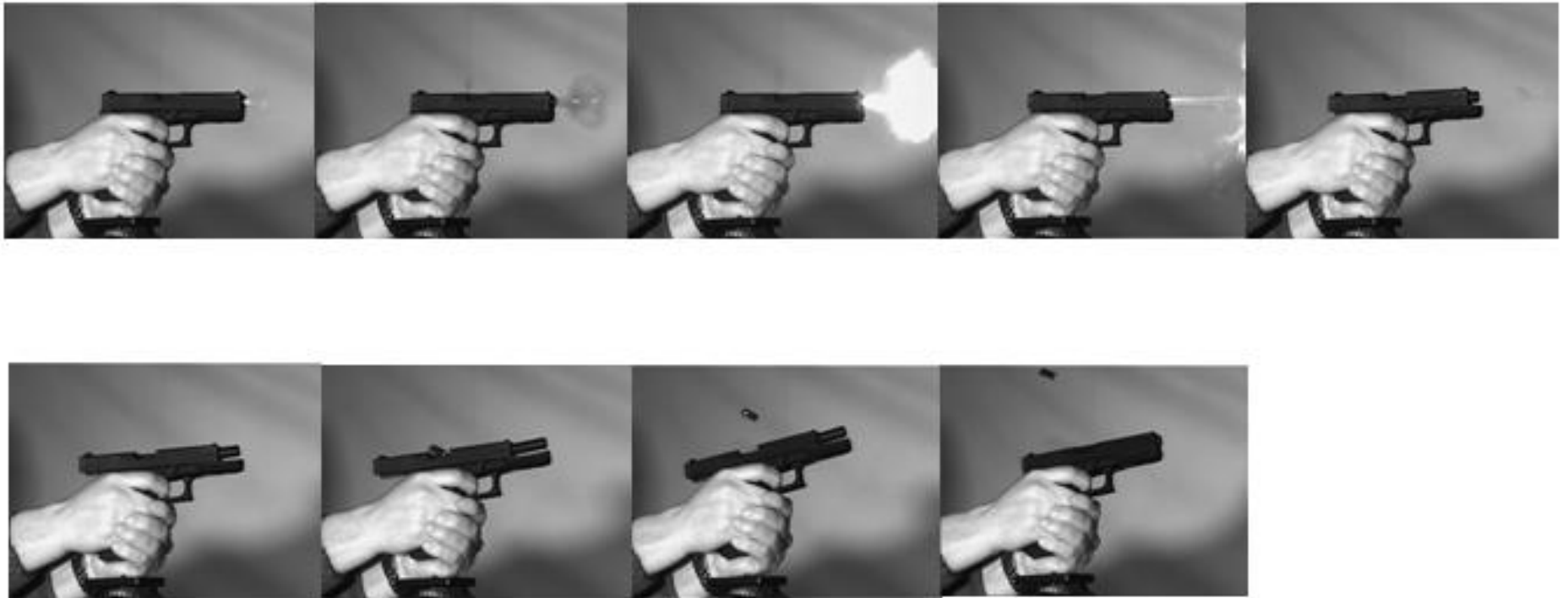
Figure 38: Still frames taken from fast video footage of a Glock 26 discharge (close framing). Settings of the fast video equipment were; frame rate 10000 fps, exposure time 100usec.
