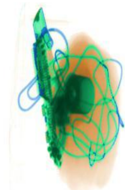
Fig. 3.15. Sample perspective colour images produced by the multiple view line-scan X-ray image intensifier system.
