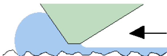
Figure 6.3.2.1 Diagram of how bird type applicator applies coating.
