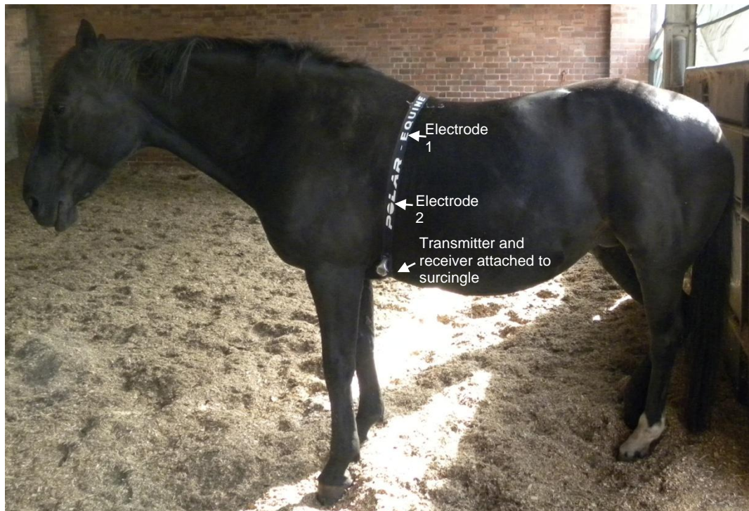
Figure 2.5 Horse wearing heart rate monitor. Transmitter and receiver position and position of electrodes in the region of the upper left thorax and the ventral midline are labelled.
