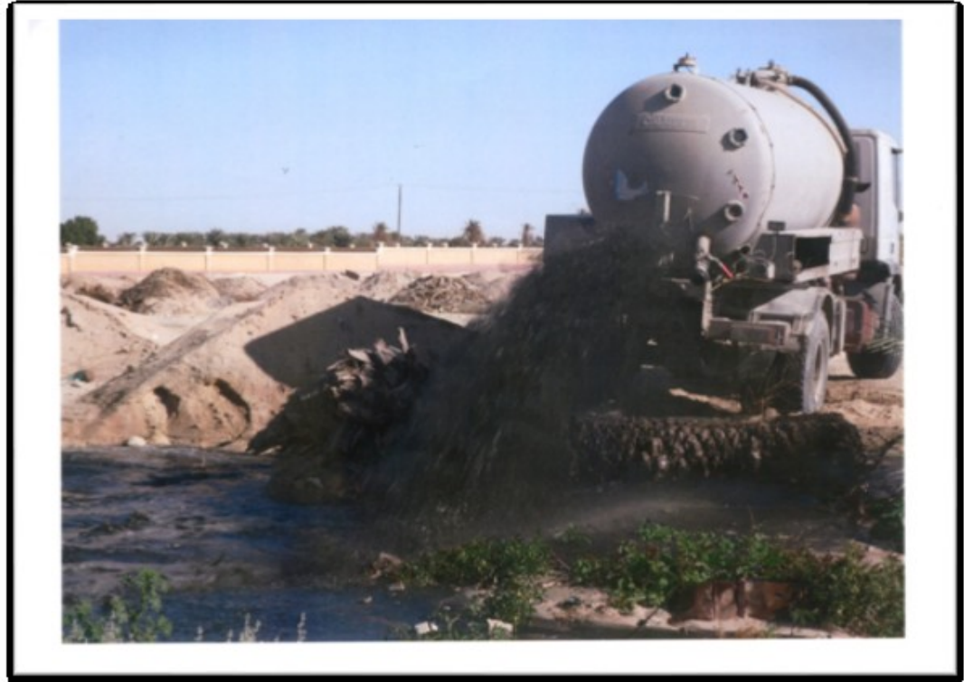
Figure 20: Evidence of unregulated discharge of sewage from septic tanks to the ground surface. Approximately 1 km from the residential area of Alwihat. The wall in background of this photo is a farm boundary (photo by the author, 2010).
