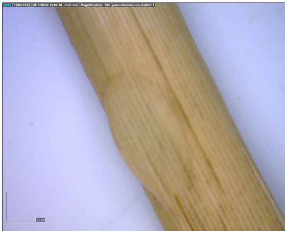
Figure V.34: External surface of straw. Water bead: hydrophobic nature
