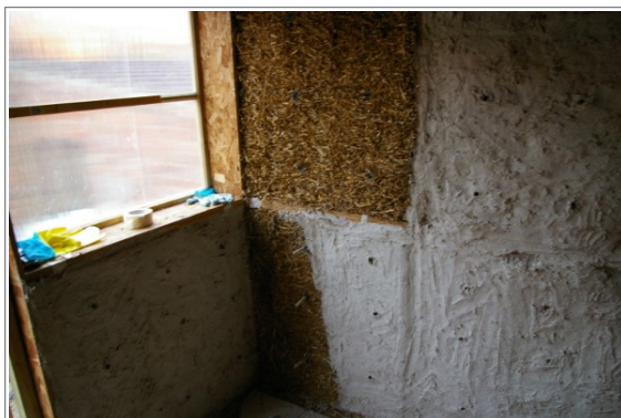
Figure V.15: Holes marked for insertion of Balemaster probe from rig interior.
