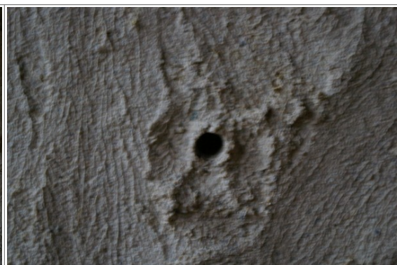
Figure V.16: Hole for insertion of BM probe.
