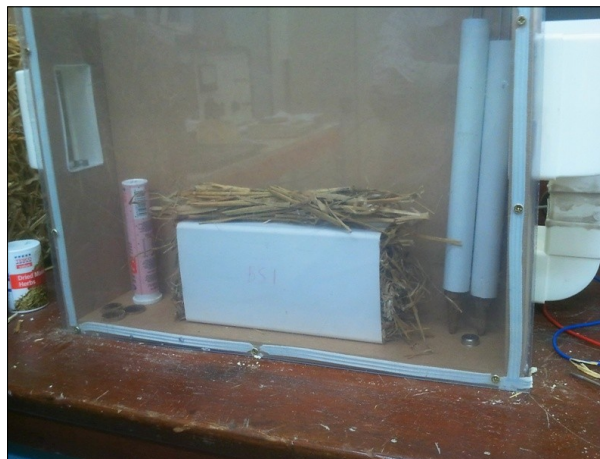
Figure VI.11: Environmental Chamber with Containment Sleeve Sample
