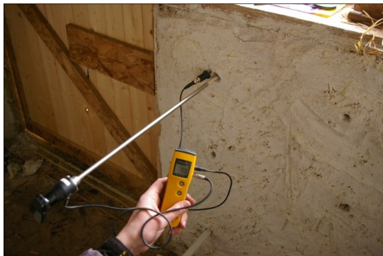
Figure V.14: Monitoring of Module-block with Balemaster showing holes to interior side of render
