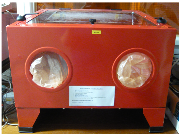
Figure IV.5: ‘In-house’ dry box used for separate density viscosity measurements.
