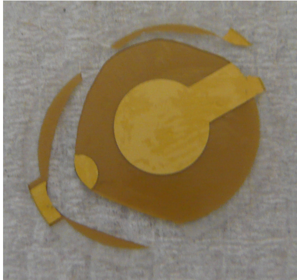
Figure V.10: A failed Quartz Crystal: the pressure within the lab-on-a-chip device has exceeded the crystal's limit which has cracked around its weakest point.
