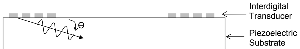
Figure II.14: Image of Surface Skimming Bulk Wave (SSBW), showing shear horizontal polarisation propagating at a shallow angle \theta , down into the bulk of the crystal.
