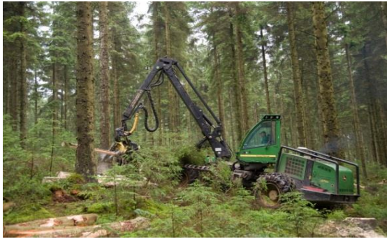
Figure 19: A harvesting machine. Trees are felled, de-limbed and cut into logs in a single operation.
