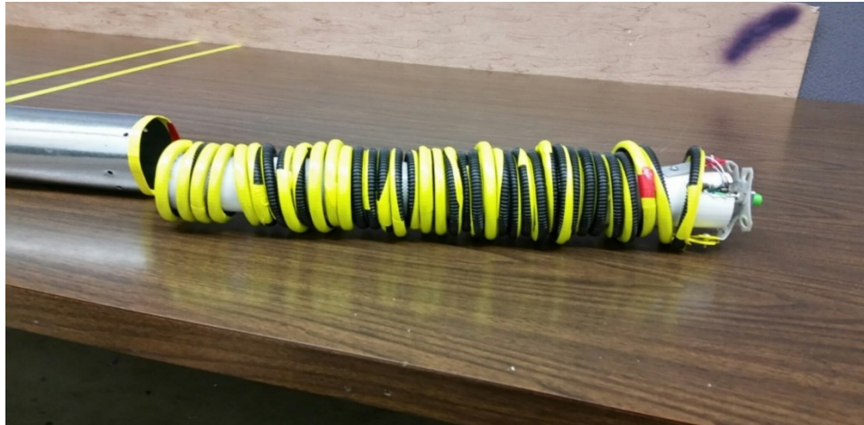
Figure A4.10: Assembly of Fiber optic Coil on Central PVC Pipe
