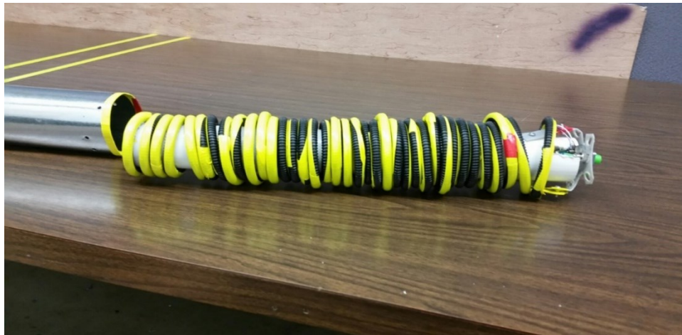
Figure 4.1: Assembly of Fiber Optic Coil on Central PVC Pipe
