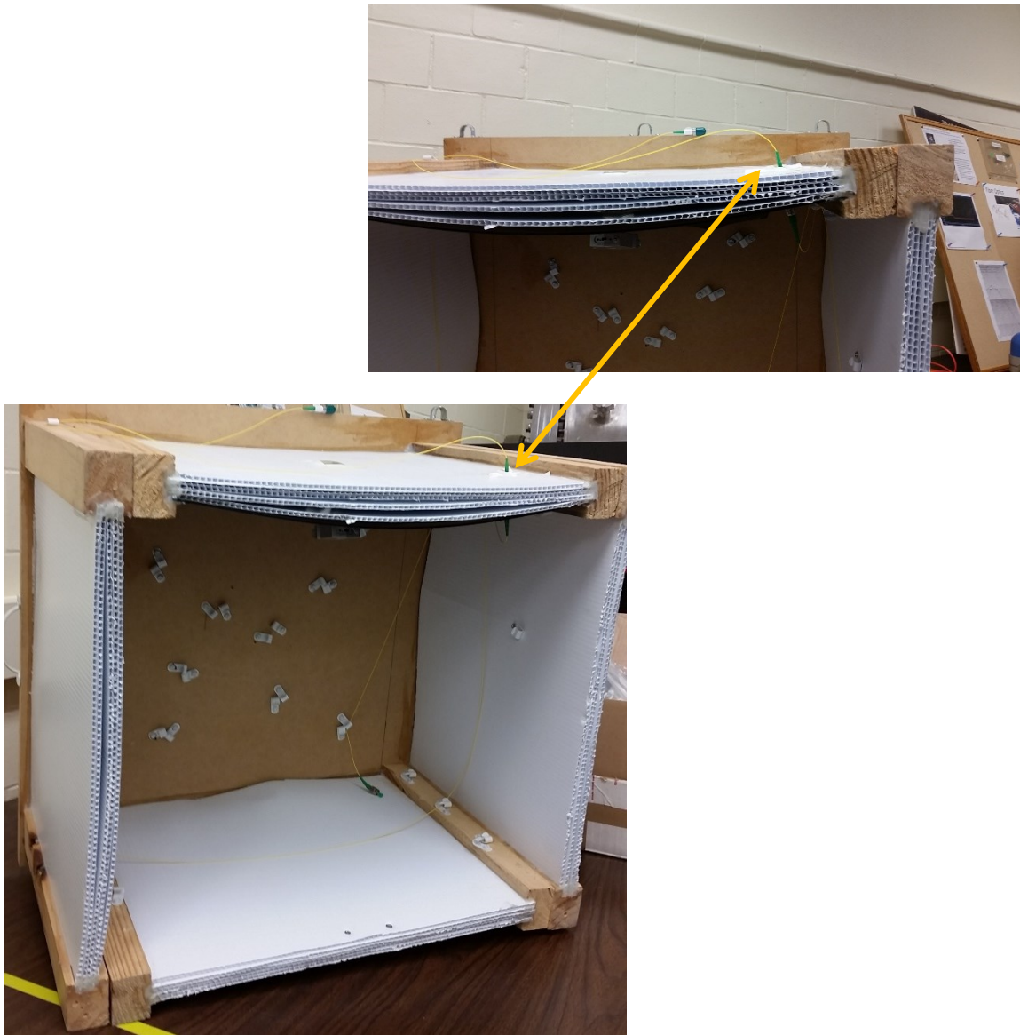
Figure A3.7: Fiber Optic Spiral and Jumper Connection
