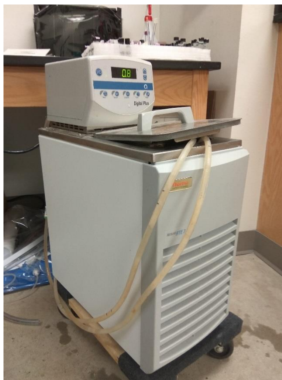
Figure 3-7: Thermo Scientific, Neslab RTE 7, circulating bath
