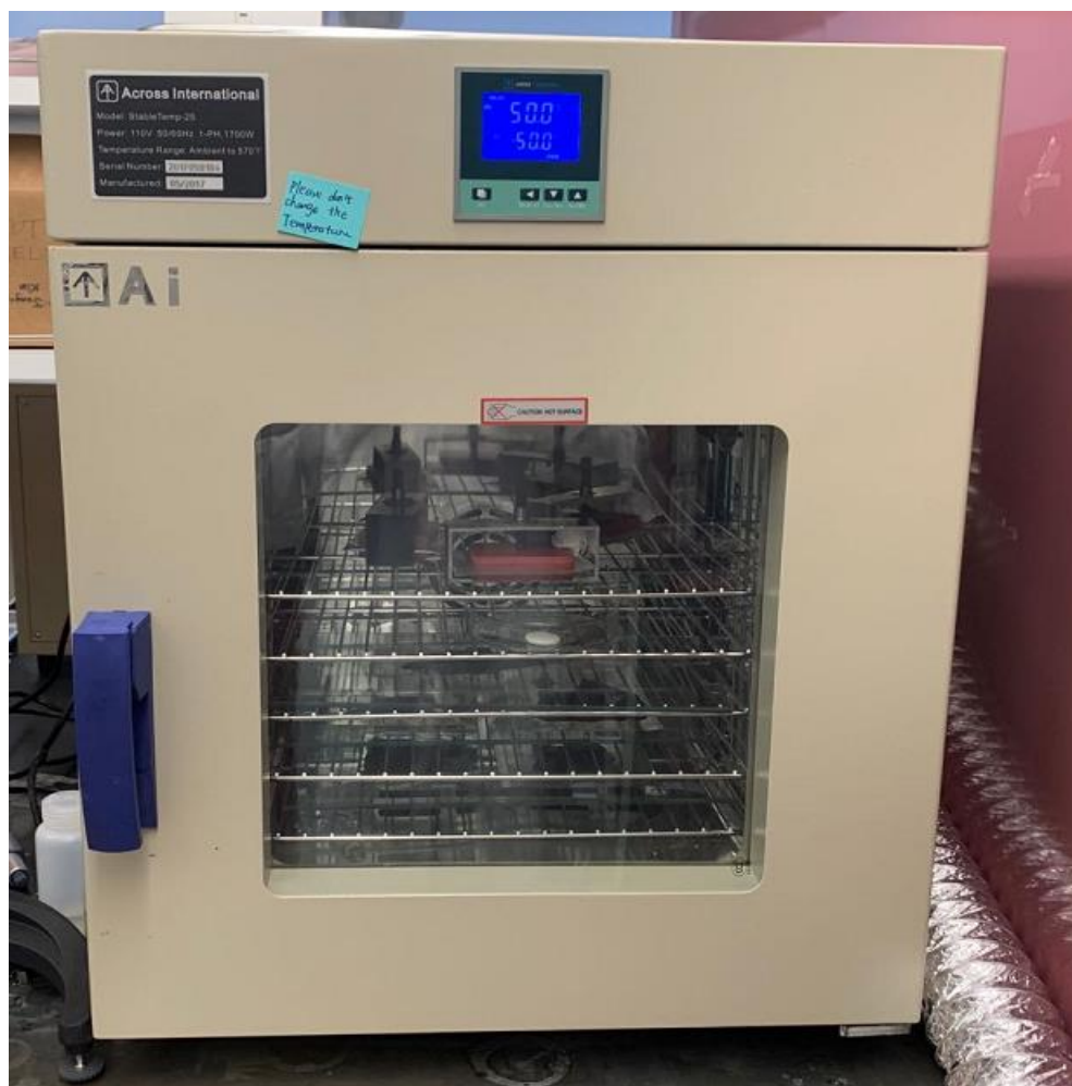
Figure 4: Vacuum Oven for drying the anode material
