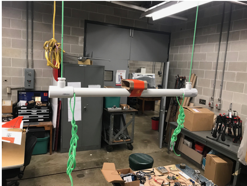
Figure 3.3: Modified Bifilar Pendulum Setup
