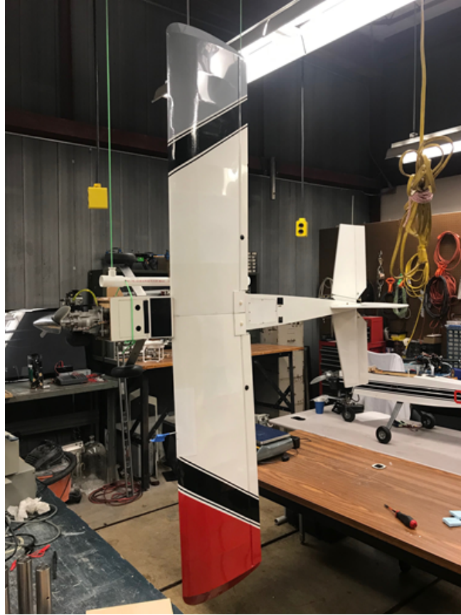
Figure 3.9: Mentor V1 in I_{yy} Testing Configuration
