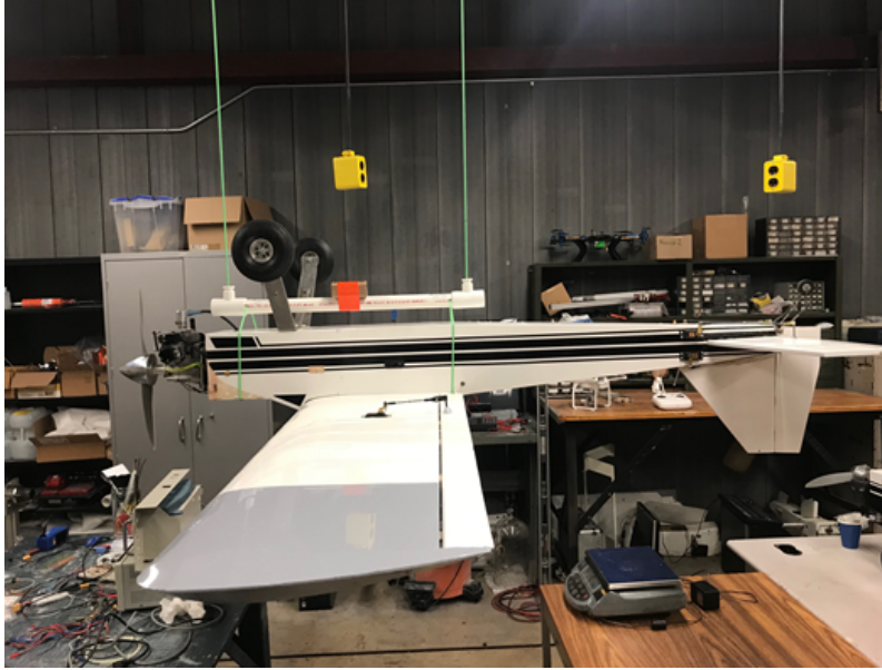
Figure 3.11: Mentor VI in I_{zz} Testing Configuration
