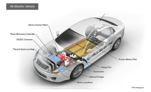
Fig 2.2 Key components of an all-electric vehicle. (Source: afdc.energy.gov)
