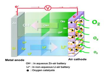
Fig 2.9 Schematic structure of a metal-air battery.
