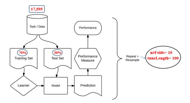
Fig. 5.5 Machine-learning algorithm framework.
