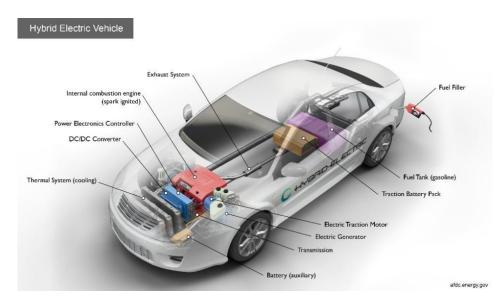
Fig 2.4 Key components of a hybrid electric vehicle. (Source: afdc.energy.gov)
