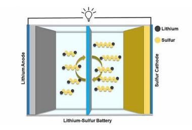
Fig 2.8 Schematic structure of a lithium-sulfur battery. (Source: https://aip.scitation.org)
