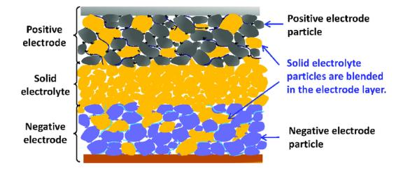
Fig 2.6 Schematic structure of a solid-state battery. (Source: [20])
