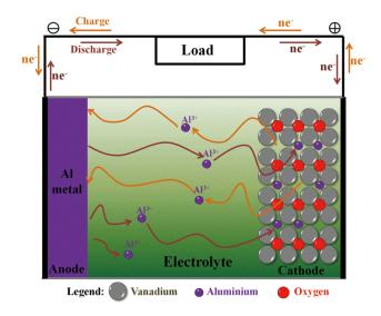
Fig 2.7 Schematic structure of an aluminum-ion battery. (Source: [23])
