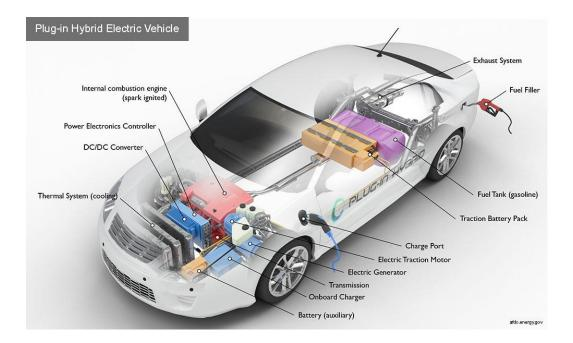
Fig 2.3 Key components of a plug-in hybrid electric vehicle. (Source: afdc.energy.gov)
