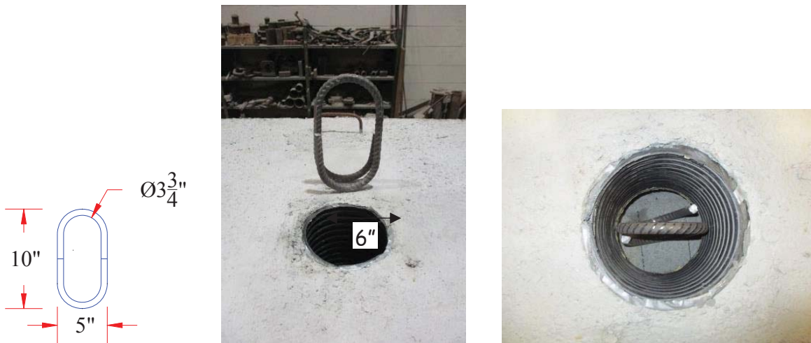
Figure 4.034: #5 Loop Bar Details and Installation.
