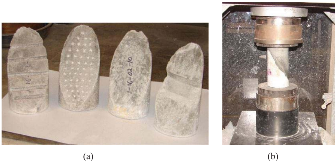
Figure 2.13: Slant Shear Test; (a) Mortar Different Roughened Surfaces and Trapezoidal Shear Key, (b) Test Setup (Harris et al. 2011)
