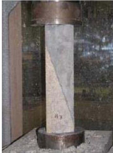
Figure 2.20: Slant Shear Test Configuration (Muñoz 2012).
