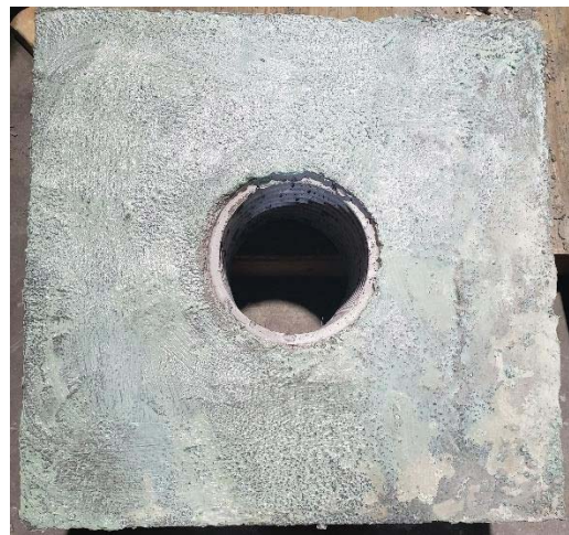
Figure 4.012: Concrete Section Preparation of Double Shear Test Specimen; (a) Removed Plastic Pipe, and (b) Applying Wax on Concrete Surfaces.
