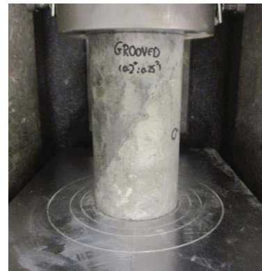
Figure 4.019: Slant Shear Test Specimen Dimensions and Test Setup.
