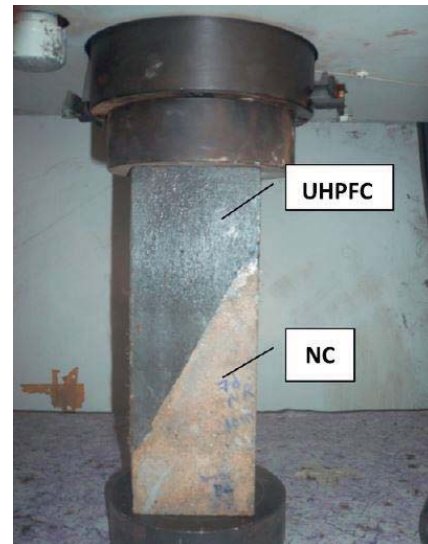
Figure 2.16: (a) Mix Proportions of UHPFC and NC, (b) Surface Textures, and (c) Test Configuration (Tayeh et al. 2012)
