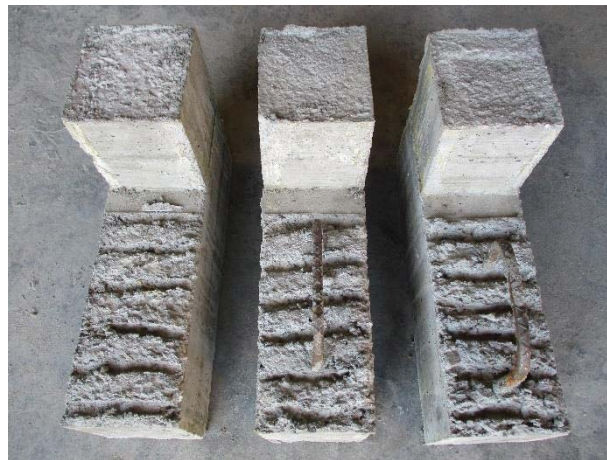
Figure 4.025: Interface Surface Roughening and Different Reinforcement across Interface; No Reinforcement (Left), 2#3 (Middle), and 2#4 (Right).
