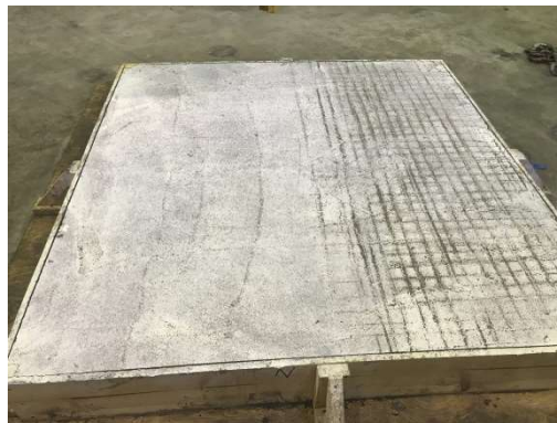
Figure 2.11 Slab 3 – Image after Scanning the Slab with GPR at 3 and 4 Hours on Curing Compound
