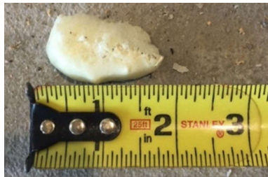
Figure 2.5 Slab 2 – Small Artificial Air Void
