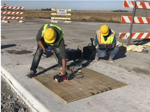
Figure 2.23 Field Experiment 2 - GPR Scanning
