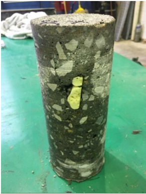
Figure 2.17 Slab 3 - Core 8 (Large Void)
