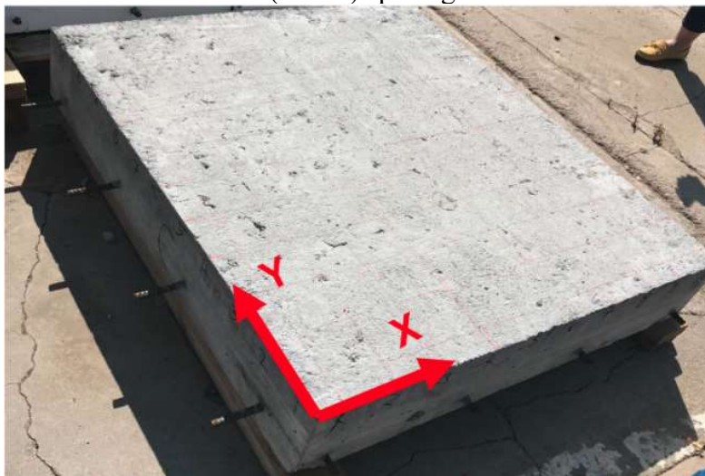
Figure 2.1 Slab 1- Specimen Photo and Scanning Axes
