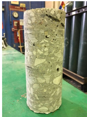
Figure 2.19 Slab 3 - Core 13 (Compressed Air)
