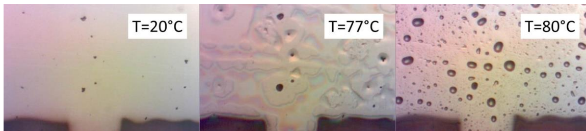
Figure 7. Still frames from a movie of a VDF oligomer thin film on a Pt/Co electrode being heated. For reference, the movie is taken at the location where the thin strip (bottom of the still frame) meets the square pad (see figure 1) of the bottom electrode. The film undergoes a dramatic change around 75 °C. At 80 °C, the pyroelectric signal disappears and bubble-like features appear on the surface of the film and remain even after the film is cooled back down to room temperature.
