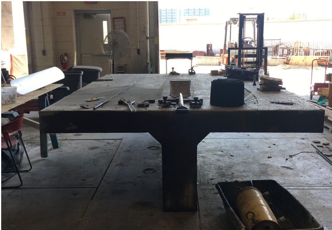
Figure 4.10: Proposed Standard County Bridge Section after Construction
