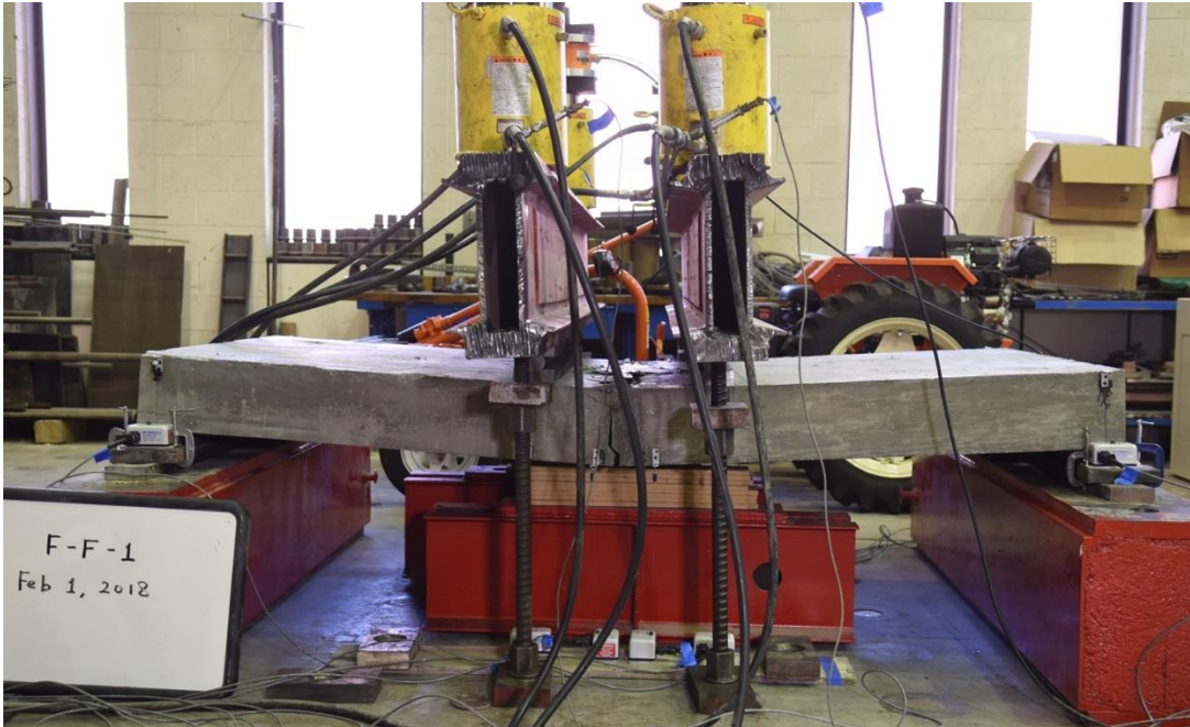
Figure 3.13: Concrete Crushing at Top (Specimen F-F-1)
