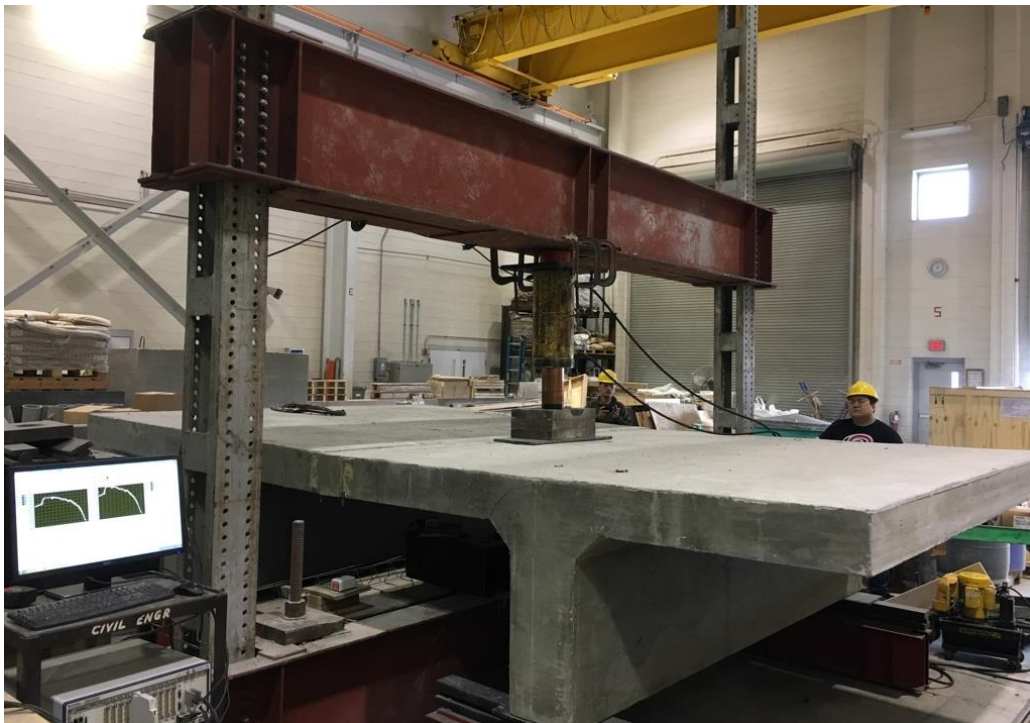
Figure 4.21. Test Setup and Loading of Specimen F-R-SHPC
