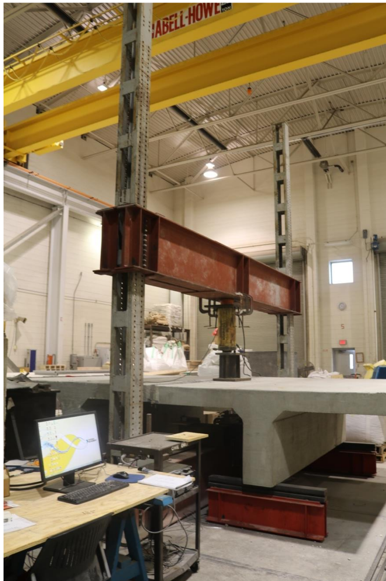
Figure 4.12: Full-Scale Specimen Test Setup
