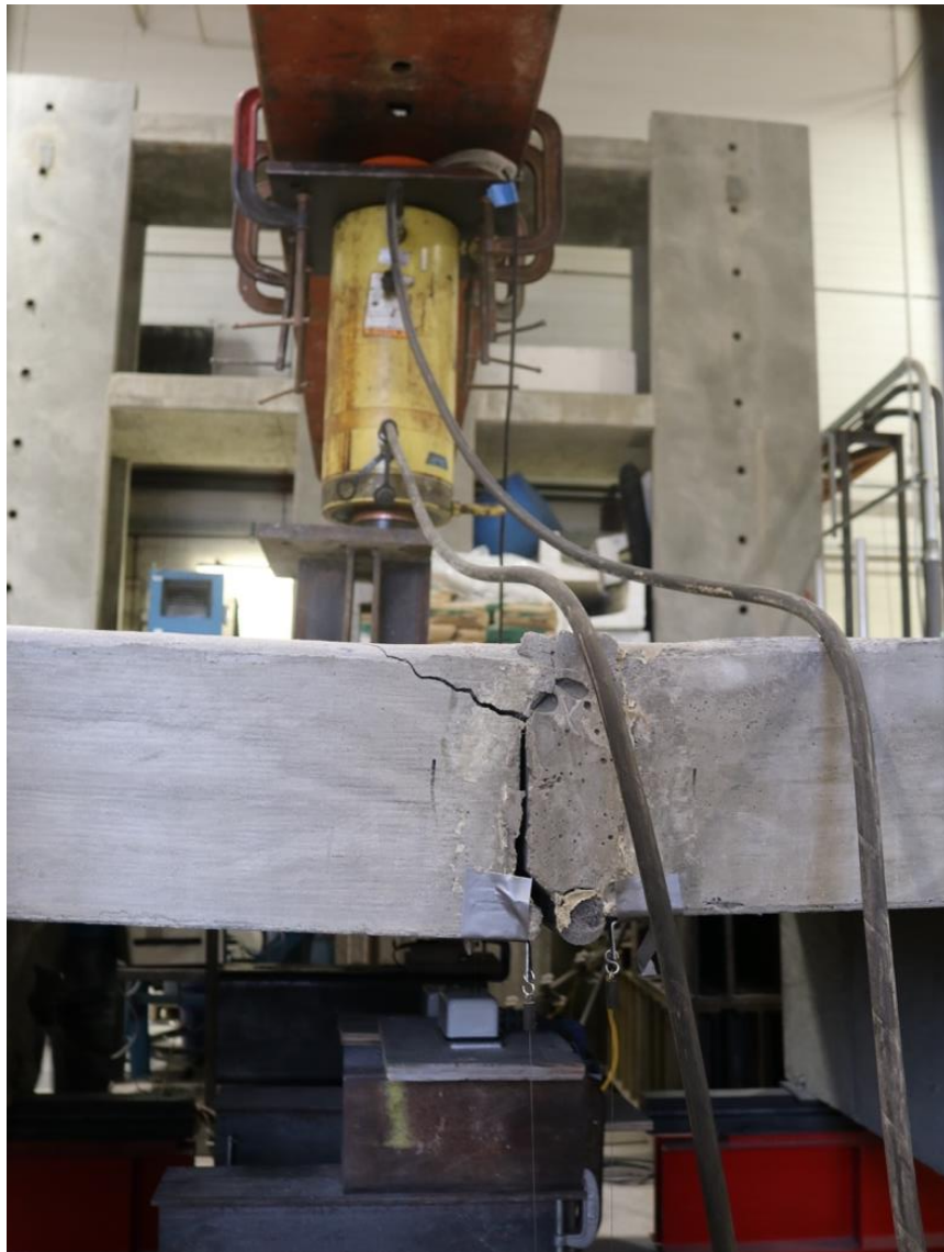
Figure 4.14: Close-up view of the Grouted Joint (Specimen F-M)
