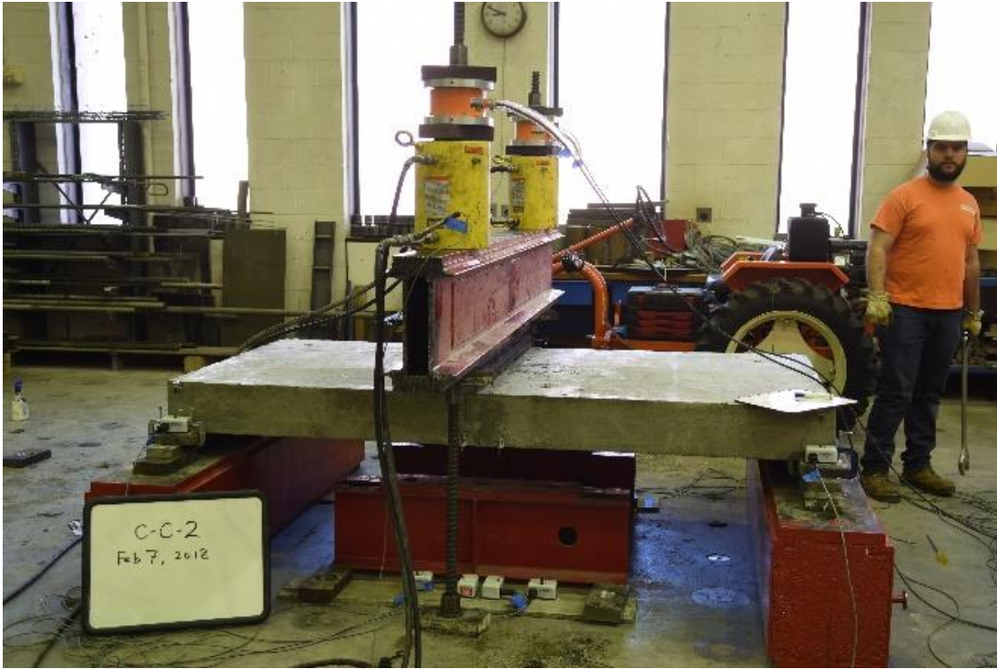
Figure 3.30: Three-point Bending Test Setup (Specimen C-C-2)
