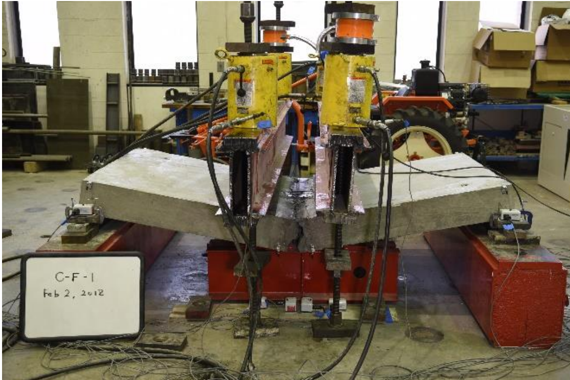
Figure 3.28: Specimen C-F-1 at Failure
