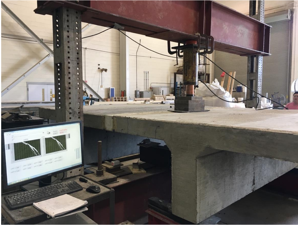
Figure 4.19: Test Setup and Loading of Specimen F-L-UHPC
