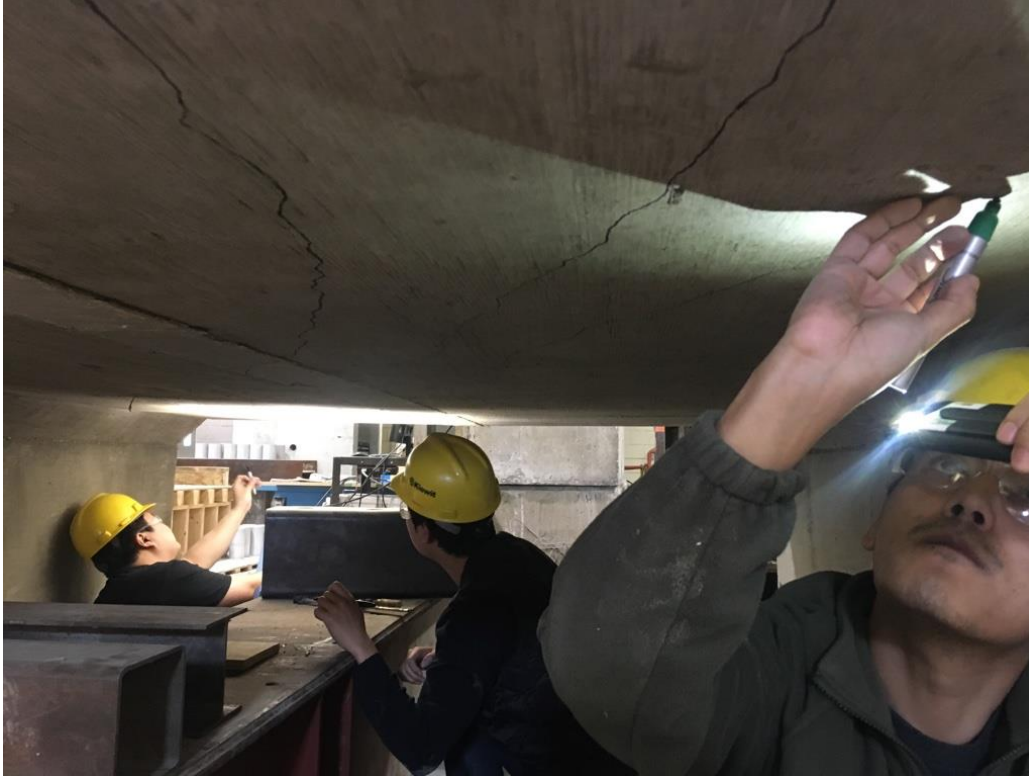
Figure 4.22. Crack Mapping and Failure of Specimen F-R-SHPC
