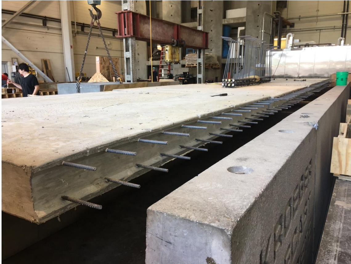
Figure 4.11: Test Specimens with Short Splice Length
