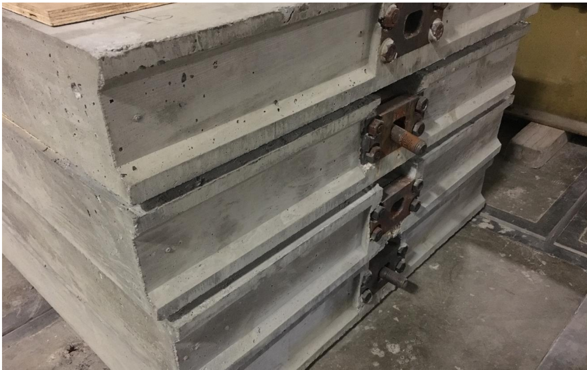
Figure 3.7: Slab Panels with Mechanical Joints
