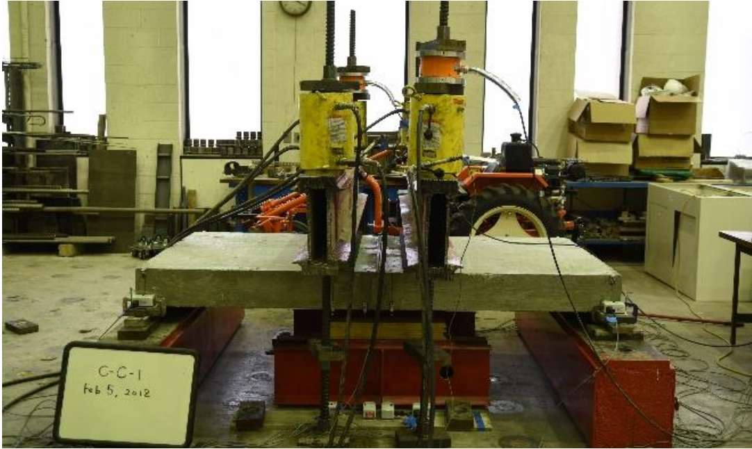
Figure 3.18: Four-point Bending Test Setup (Specimen C-C-1)
