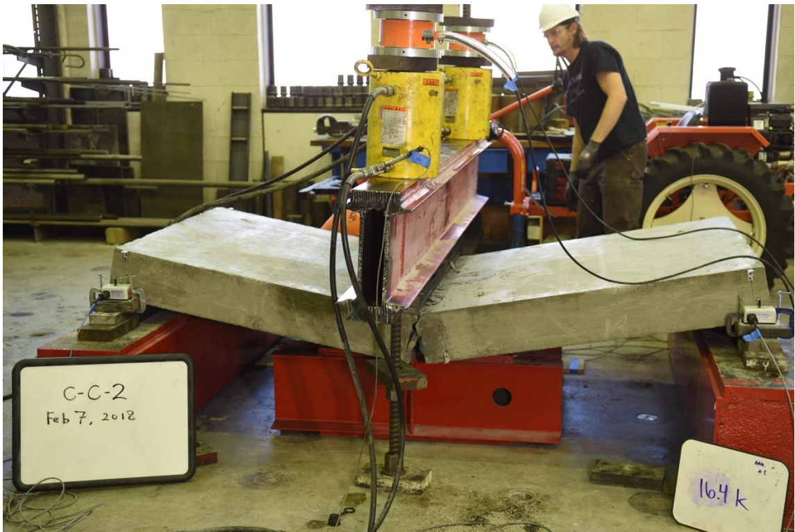
Figure 3.33: Specimen C-C-2 at Failure
