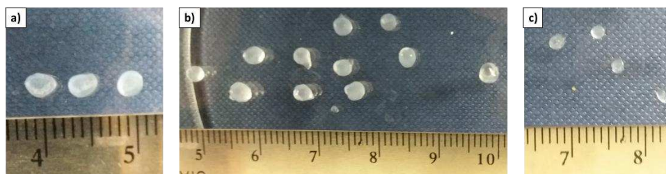
Figure S4. DBS-CONH 2 /alginate two-component gel beads prepared by addition of 20 \mu\text{L} (a and b) and 5 \mu\text{L} (c) volumes into a CaCl 2 solution (5%). A ruler was included to show the diameters.
