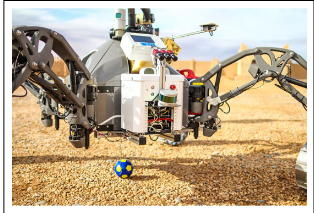
Figure 3. The HCRU engineered by DLR Institute of Robotics and Mechatronics, includes two monochrome cameras, a color camera, lidar, and IMU. In the figure, the device is mounted on the side of DFKI's SherpaTT robot. HCRU: Handheld Central Rover Unit.
