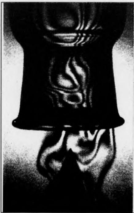
Figure 26: Double-exposure interferogram of CO 2 venting from a glass column
