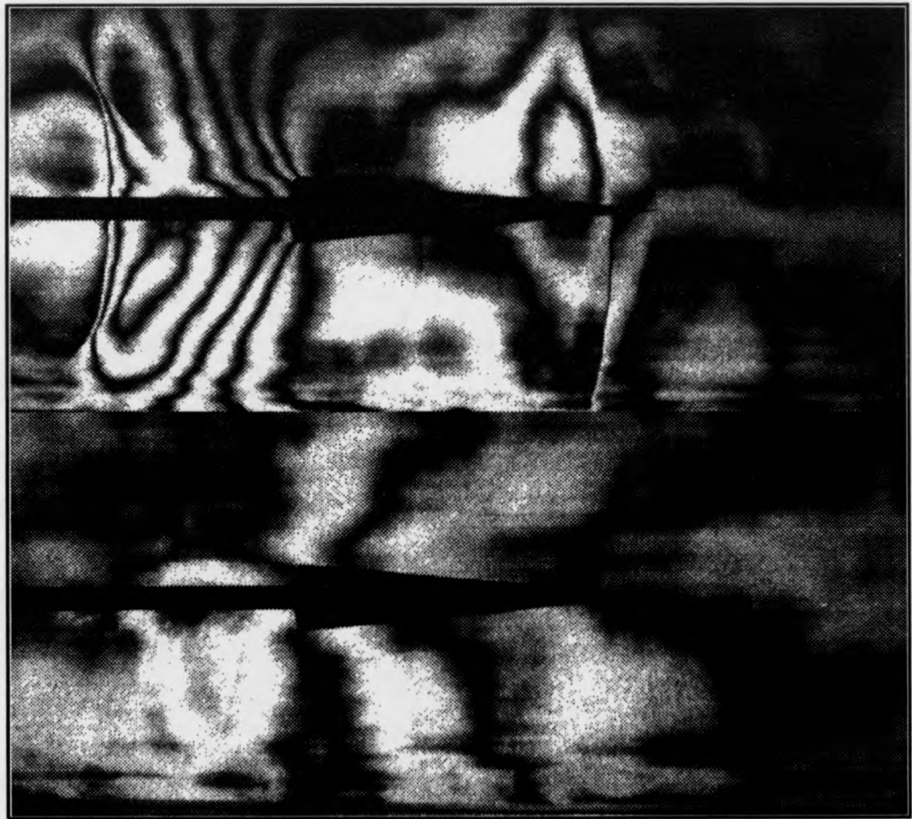
Figure 88: Transonic flow over a cone with freestream Mach numbers of 1.13 and 0.99
