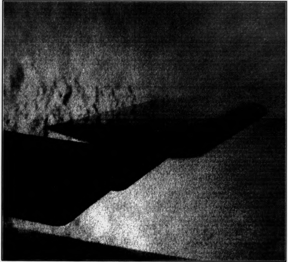
Figure 18: Formation of turbulent features in a region of separated flow
