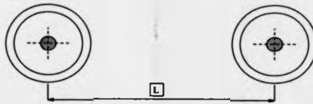
Figure 5.3: Annular template containing data points and reference centres within position tolerance.
