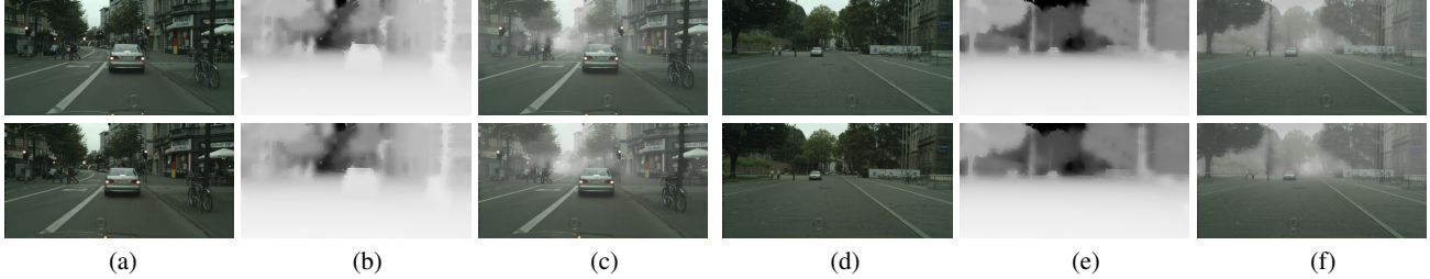
Figure 3. Example images of our generated Stereo Foggy Cityscapes dataset. Top row: left images, Bottom row: corresponding right images. (a) and (d): clear stereo image pairs; (b) and (e): transmission maps; (c) and (f) foggy stereo image pairs.
