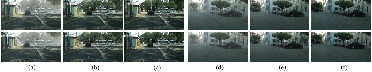
Figure 5. Qualitative results on Stereo Foggy Cityscapes val Dataset. (a) and (d) stereo foggy images. (b) and (e) stereo haze-free images dehazed by BibNet. (c) and (f) ground truth (stereo clear images).
