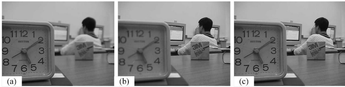
385 (a) (b) (c) 386 Fig. 6. A pair of multi-focus images that are used to test the impacts of different parameters on the fusion performance in the 387 proposed dictionary learning method and the proposed fusion method. (a) Focus on the left part; (b) Focus on the right part; (c) 388 'Ideal' fused image.
