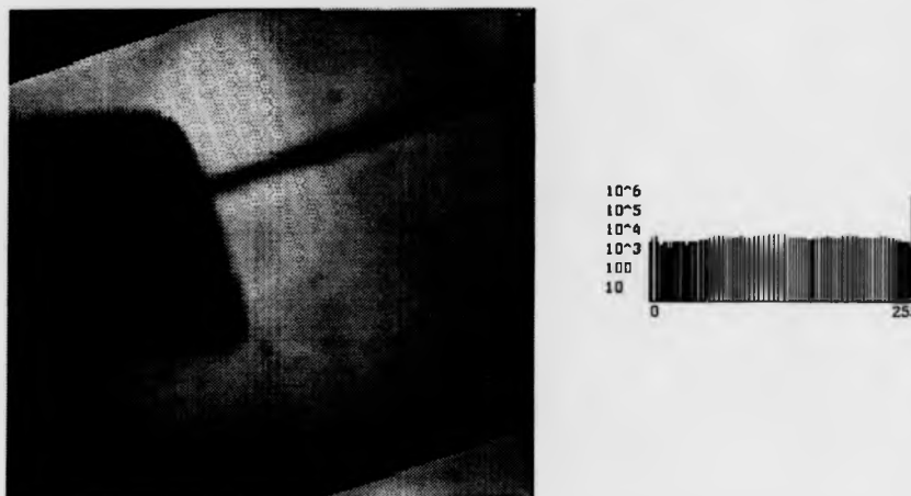
Figure 4.12: (a) Result of processing Figure 4.11 with the histogram equalisation algorithm, and (b) its histogram.
