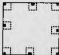
Figure 5.10: Pixels around the edge of the image and the regions they are assigned.
