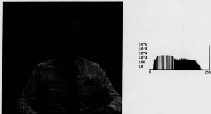
Figure 6.12: (a) Result of applying the smoothed histogram equalisation algorithm to Figure 4.6 with \lambda = 0.3 and, (b) its histogram.
