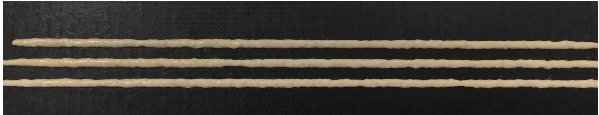
309 310 Figure 8: Extrudability test showing three printed lines of material.
