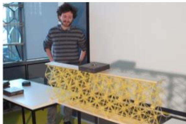
Figure 6. Open-web truss (2013) – Students were asked to design and build a truss that was 1400mm long and 330mm deep that could support a centrally positioned load of 20kg. (The size of the truss was based on the ground floor fenestration of the UoW Marylebone building.)
