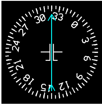
Fig. 2-13. ADF Indication to NDB
