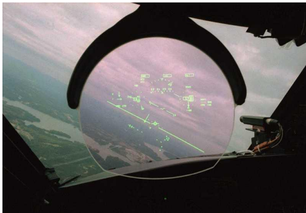
Fig. 2-10. Head-Up Display Combiner
