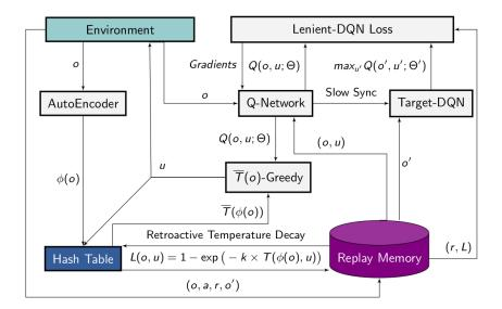
**Figure 6.1:** Lenient-DQN Architecture. We build on the standard DQN architecture [217] by adding a lenient loss function (top right, see Section 6.2.2). Leniency values are stored in the replay memory along with the state transitions; we cluster semantically similar states using an autoencoder and SimHash (bottom left), and apply our retroactive temperature decay schedule (TDS, Algorithm 6). Actions are selected using the  $\overline{\mathcal{T}}$  (o)-Greedy exploration method.
