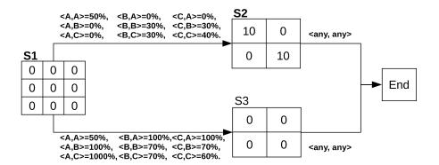
Figure 5.7: Relative Overgeneralization 3 State Transition Diagram (Illustration is adapted from Wei and Luke [223]).
