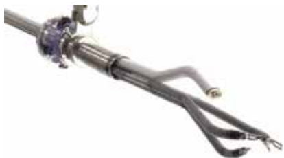
Figure 4 Intuitive Surgical SP 1098 single port articulated endoscope and instruments. (Image credit Rassweiler et al, 2017 25 )
