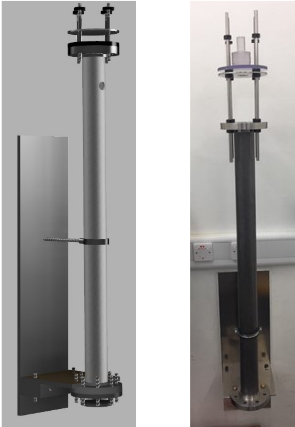
Figure 7.15: CAD of the rig in wall mount (left) with photograph of the rig in wall mount (right). The projectile is seen upon the top plate on the right (seat not pictured).
