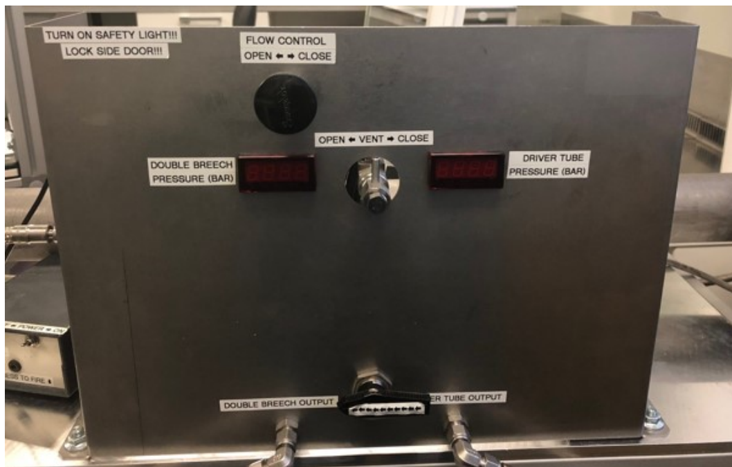
Figure 7.6: Shock tube control panel used to control input pressure of compressed air. Only one of the lower outputs is utilised.
