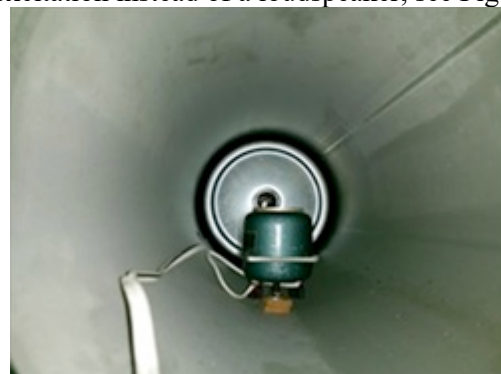
Figure 4: Vibration shaker mounted inside the pipe
