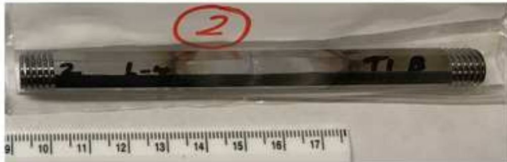
Figure 1. Sample TiB-B2 after DB. The area of the joint is in the middle of the rod. Slight oxidation is observed at about 15 mm distance on both sides from the interface between bond samples
