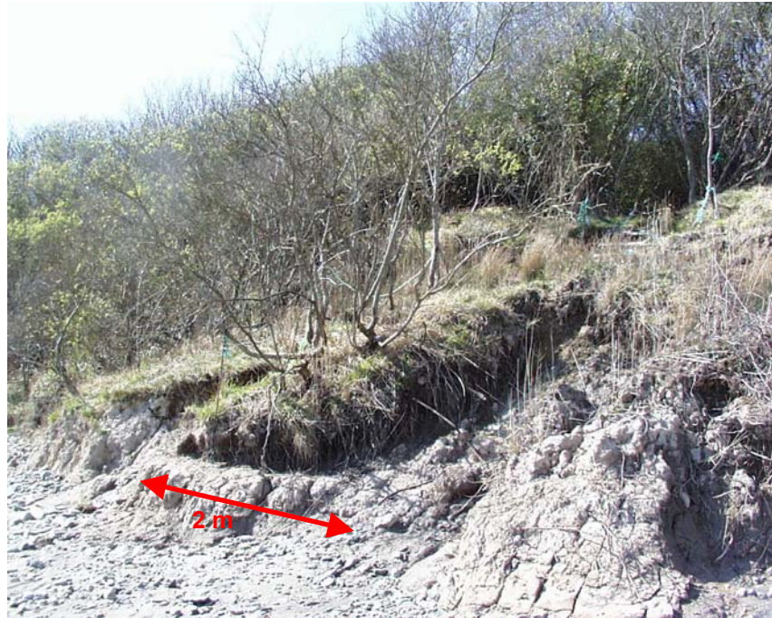
Figure 9. Exposure of disturbed soft to firm, light grey to light brown sandy clays at [224031 328306].
