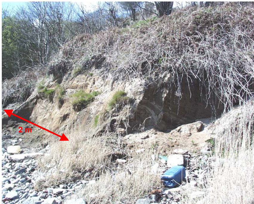
Figure 8. Exposure of soft, light brown to dark grey laminated, fine grained sands looking NW at [223973 328254, z1.5]. Although intact laminations could be seen in the exposure it is thought that the material had been emplaced as part of a slope movement.
