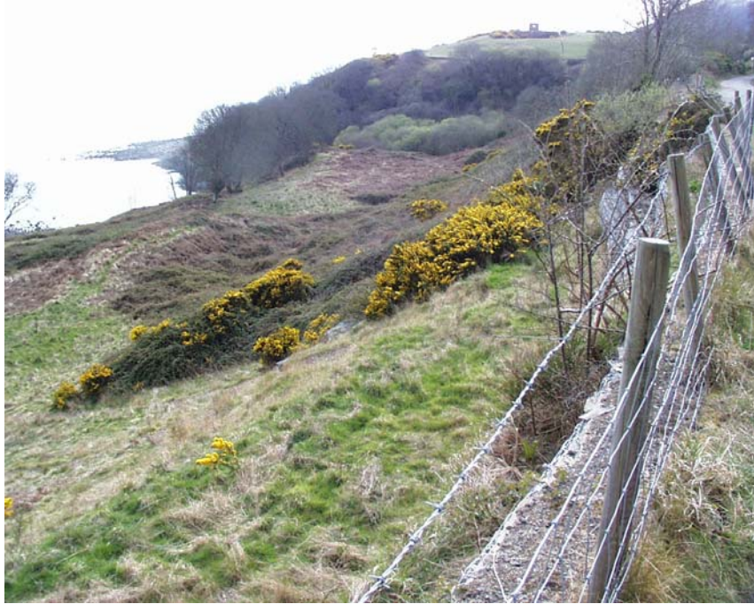
Figure 21. Distress to the fencing immediately southeast of Sarn y Plas. This photograph, facing towards the southeast is a further illustration of topography interpreted as the back-tilted blocks of rotational landslides.
